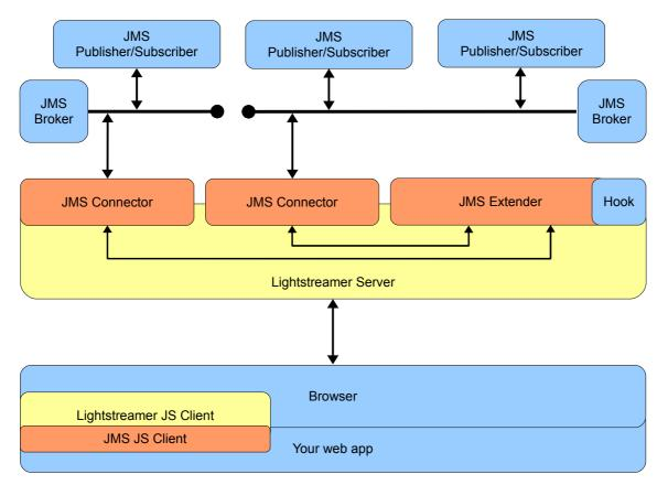
The diagram above shows the big picture of the JMS Extender architecture, with color-coded boxes depending on which layer they belong to:
