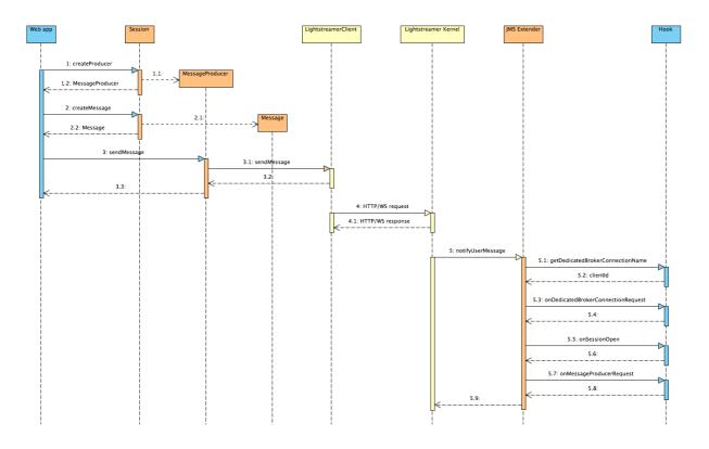
Similarly to the previous diagram, creating a message producer on the client side does not deliver any notification on the extender side. Only when a message is actually sent the extender is made aware of the operation and calls the hook's methods accordingly.
