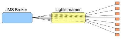
JMS Extender without connection offloading
