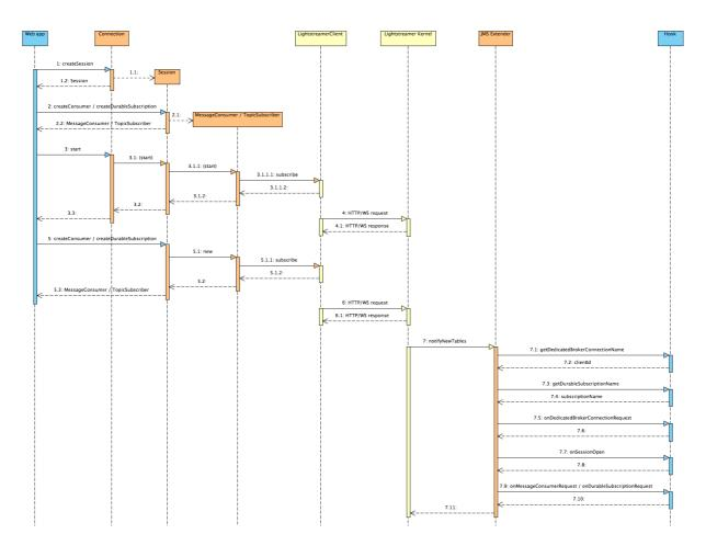
As per JMS specification, creating a message consumer is not enough to start receiving messages: its connection must be started too. When this happens on the client side, the message consumer is actually activated and on the extender side the hook's methods are called accordingly. Message consumers created subsequently will be activated immediately.
